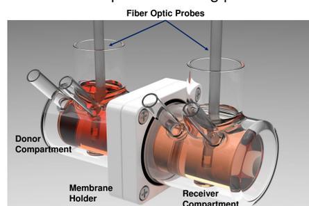
Figure 2. A fragment of the  $\mu$ FLUX apparatus showing a pair of the donor and receiver chambers. FO probes attached to the  $\mu$ DISS Profiler monitor concentrations in the donor (left) and receiver (right) compartments. The chambers can be separated by PAMPA, cell-based (Caco-2 or MDCK), dialysis, or other types of membranes mounted in the Membrane Holder.
